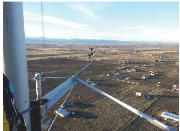
Figure 4: Anemometer and vane on the northwest 150m boom on BAO.
